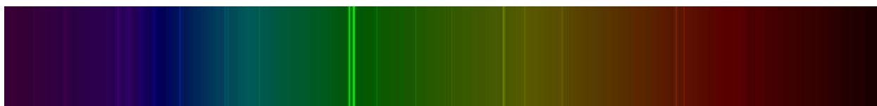
Figure 5. Magnesium Emission Spectra
